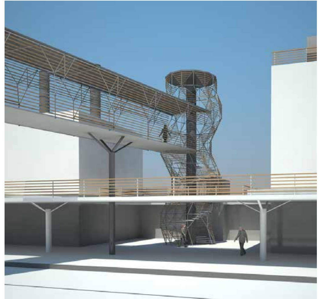
Another view of one of the connecting bridges.The Use of lattice structures and the particular form of the scale are a tribute to the industrial tradition of the city of Milan. The Porta Garibaldi Station was, in fact, designed by Eugenio Gentili Tedeschi,( professor and architect very influenced by the thematic of industrialization related to architecture)and located in the "Isola Garibaldi"district in Milan,where,during the first half `of the last century, some of the first main factories were erected.
