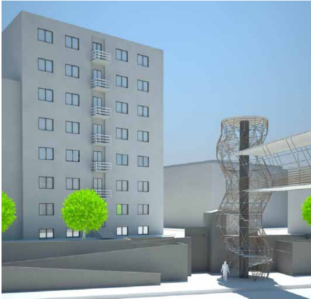
View from the rails' level of one of the bridges that connect Via Ferrari to Isola DIistrict. The bridge built by a reticular structure, represents the continuation of the balconies of the "Rustici Comolli" house(Visible in the background), built in 1935 by Giuseppe Terragni.One of the first examples of Italian Rationalism This final result was a modern reinterpretation of the house railing typical of rural areas in Milan.
